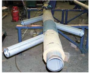
Ireland, FW SAFETY PIPING for contaminated waste water, DN 100/200, 150/200, 150/250, 100° C, 6 bars, inner and encasing pipes of stainless steel
