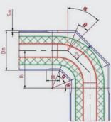
SIS pipe bend with multiple segments for large dimensions
